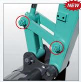
The arm-end and boom-arm joint are fixed with castle nuts. The reduction of horizontal tolerance is achieved.
