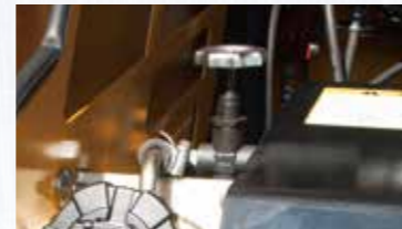
▲ Emergency stop valve for lowering the bed
