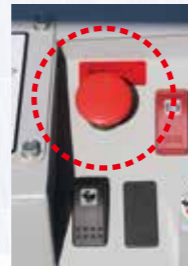
▲ Emergency engine stop button
