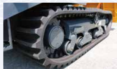
▲ Triangle-shaped crawler frame
